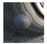
Potholes can cause serious tire damage.
