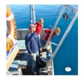
The Secchi disc is lowered into Lake Tahoe for one of several readings. Photos/TERC
