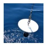
The Secchi disc is the main means to measuring lake clarity.
