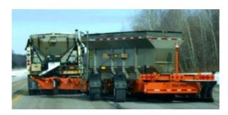
The tow plow allows more snow to be removed at once. Photo/Provided
