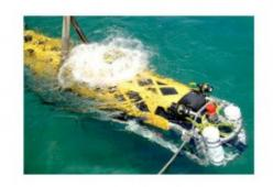
The remotely operated vehicle's vertical thrusters are tested when it was put into Lake Tahoe in early July. Photo/Ross Powell/Northern Illinois University
