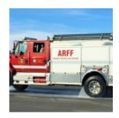
• Truckee firefighters have a new engine with wildland and ARFF capabilities. It is equipped with a 750-gallon tank, 1,250 gpm pump, 50 gallons of foam, a front bumper mounted pumpand-roll turret, a roof mounted remote operated monitor for stationary fire attack, Hurst extrication equipment, high pressure
