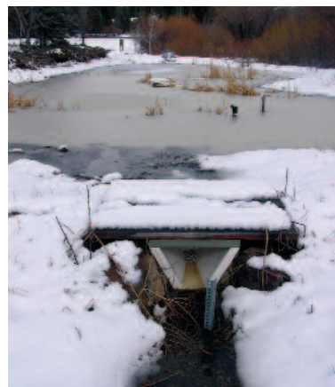
At left: Water quality projects like this one in Incline Village, NV strive to achieve multiple environmental benefits for Lake Tahoe. At right: Flow measurement device at Village Green Pond, Incline Village, Nevada.
