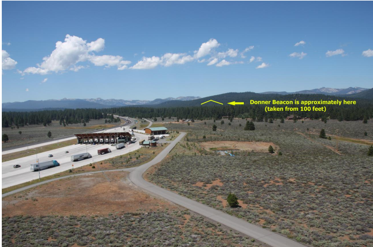
Figure 6.1. Ridgeline Blocking Line-of-Sight between the Agricultural Inspection Station and Donner Beacon (photo taken from 100' above ground surface)
