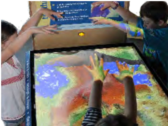
The new Interactive Sandbox exhibit captivates young and old visitors alike with evolving color contours that reflect the sculpted sand surface, and water flow simulations showing the passage of floods through the created watershed.
