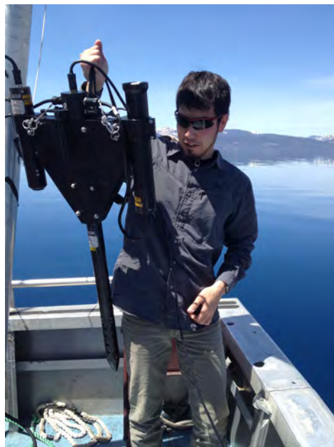
Radiometric profiles are taken regularly to calibrate the buoy sensors.
